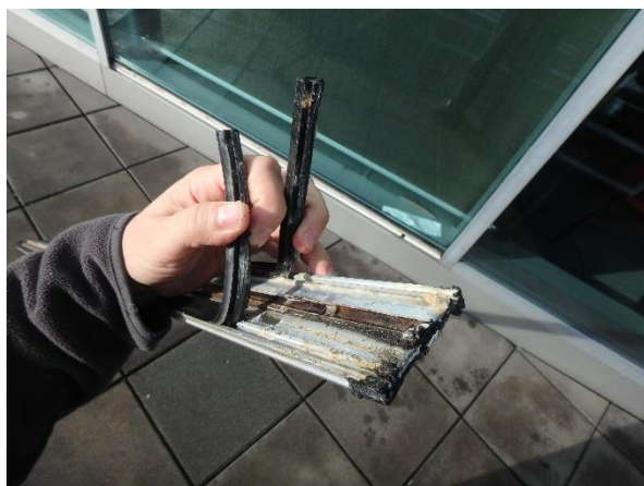
Photo 3.1-3: Aged and shrunken pressure plate gaskets. The gaps at the gasket ends allow water into the glazing cavity.
