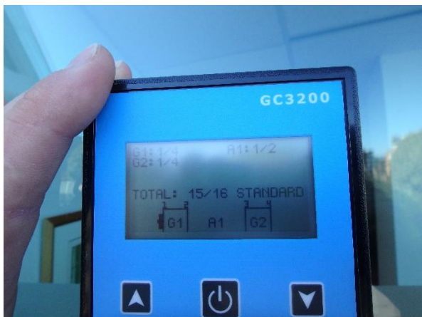
Photo 3.1-19: The current glass configuration is 1/4" clear glass – 1/2" space – 1/4" clear glass.
