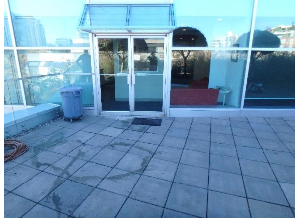
Photo 3.3-2: Membrane water testing in front of the southernmost swing door – 3 rd floor terrace.
